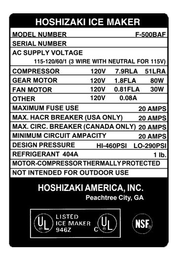
See the nameplate for electrical and refrigeration specifications. This nameplate is located on the upper right hand side of the rear panel.
